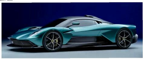
The production car is a hybrid with a V8 engine that produces 740 BHP. Aston says the engine is the 'most advanced, most responsive and highest-performing' it has ever used. The exhaust system has active flaps and high-mounted tailpipes to give a satisfying bark to match its bite.
