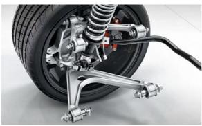
Another type used in some rear-wheel drive cars is the Chapman strut, named after Lotus founder Colin Chapman. This design features a coil spring surrounding a shock absorber, and the tubular shaft's lower connections to the body are a drive-shaft and radius arm. The coil-over shock absorber is a unit that encircles a telescop-
