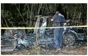
firefighters Eight eventually spent seven hours putting out the fire. They also used up 28,000 gallons of water, the volume the Woodlands Fire Department normally uses in a month. By comparison, a fire in a car with a petrol or diesel engine can often be put out with about 300 gallons, well within the
