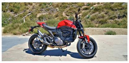
The new Ducati Monster is powered by a liquid-cooled L-twin engine of 937 cc that produces 111 BHP at 9,250 rpm and 93 Newton metres of torque at 6,500 rpm. The figures do not show large increases compared with the bike it replaces, the Monster 821 cc, but the power statistics do not tell the complete story.
