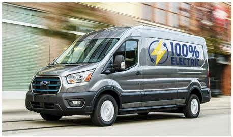
When it goes on sale, the van will be available in three roof heights and three different lengths to suit the operator's requirements. The power comes from a lithium-ion battery mounted underneath the floor. So there is no intrusion into the cargo area. The E-Transit also features an independent rear suspension which was made possible by the way its powertrain was designed, and since there is no internal-combustion engine up front, Ford has mounted the full-size spare wheel under the bonnet
